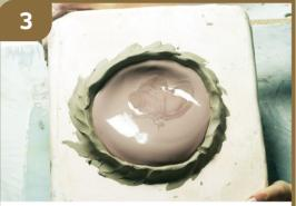
The length of time the slip is left in the mould depends on how thick the wall of the cast needs to be. A visual indication can be seen by looking at the change in colour of the slip around the edges of the mould or by moving the mould slightly to reveal the rim.
