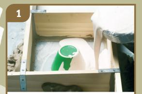
Ensure the object to be cast does not have any undercuts as this method of mould making will create a single pull mould. Place the object to be moulded on a non-porous surface. Seal all the gaps of the mould making frame with spent clay. Ballast the frame walls with extra blocks of clay. Mix the plaster (835g plaster to 1 pint of water) and pour over the object to be cast. Leave the plaster to set.
