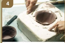
Once you have the required thickness, pour out the excess slip into a reserve bucket. Leave the slip cast shape in the mould until it has begun to shrink and release itself from the plaster walls. Trimming around the top rim can be done with a clay cutter at the leather-hard stage. The piece can then be removed from the mould and coated with decorating slip or glazes.
