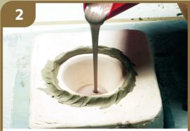
Once the plaster is dry, remove frame and object from the mould. Moulds should be left until bone dry. For slip casting, build clay edge up around the rim of the mould. Mix casting slip thoroughly then tip into the plaster mould to just above the mould top. This allows for the excess to be trimmed away neatly.
